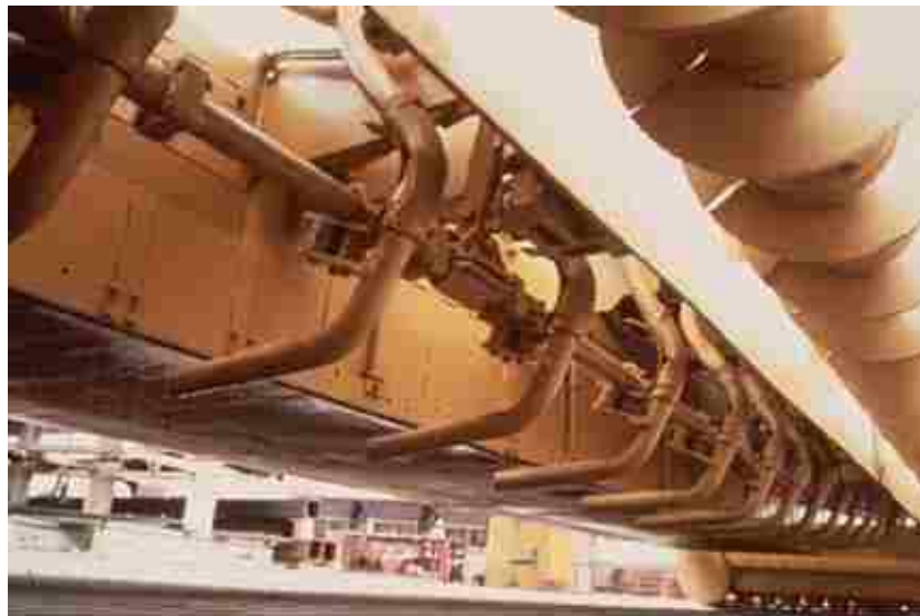
Figure 1.2 Vibrators on the underside of a paving machine [4]
