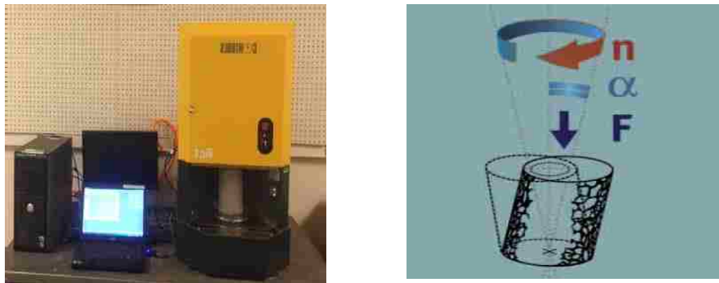
Figure 3.9 Left: Intensive compaction tester (ICT), Right: ICT compaction principal [81]
