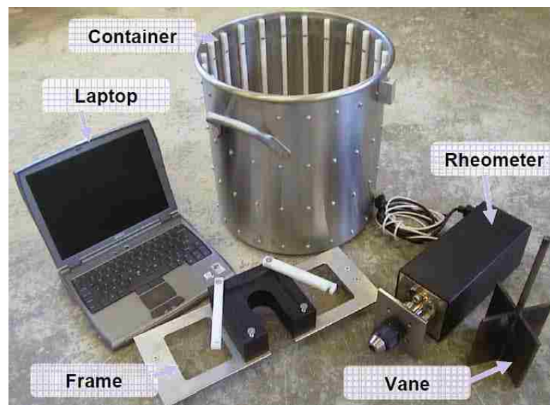
Figure 3.14 ICAR rheometer parts [95]
