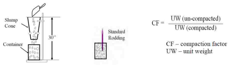
Figure 3.6 Compaction factor test setup [10]
